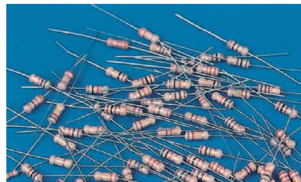
Fig. 26-7 An assortment of resistors. The circular bands are color-coding marks that identify the value of the resistance. (The Image Works)
