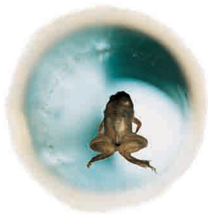
Fig. 32-13 An overhead view of a frog that is being levitated in a magnetic field produced by current in a vertical solenoid below the frog. (Courtesy A. K. Gein, High Field Magnet Laboratory, University of Nijmegen, The Netherlands)
