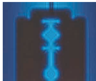
Fig. 36-2 The diffraction pattern produced by a razor blade in monochromatic light. Note the lines of alternating maximum and minimum intensity. (Ken Kay/ Fundamental Photographs )
