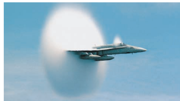
Fig. 17-23 Shock waves produced by the wings of a Navy FA 18 jet. The shock waves are visible because the sudden decrease in air pressure in them caused water molecules in the air to condense, forming a fog. (U.S. Navy photo by Ensign John Gay)
