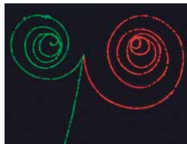
Fig. 38-10 A bubble-chamber image showing where two electrons (paths color coded green) and one positron (red) moved after a gamma ray entered the chamber. (Lawrence Berkeley Laboratory/Science Photo Library/Photo Researchers)
