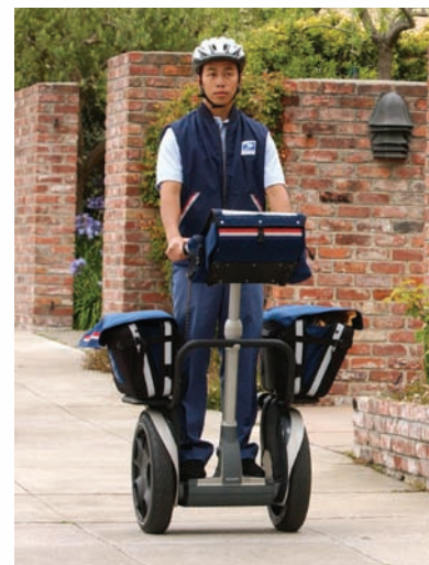
Fig. 11-1 The self-righting Segway Human Transporter. (Justin Sullivan/Getty Images News and Sport Services)
