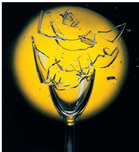
Sound can cause the wall of a drinking glass to oscillate. If the sound produces a standing wave of oscillations and if the intensity of the sound is large enough, the glass will shatter. (Ben Rose/The Image Bank/Getty Images)
