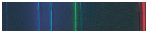
Fig. 36-25 The visible emission lines of cadmium, as seen through a grating spectroscope. (Department of Physics, Imperial College/Science Photo Library/Photo Researchers)
