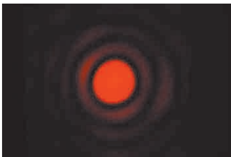
Fig. 36-10 The diffraction pattern of a circular aperture. Note the central maximum and the circular secondary maxima. The figure has been overexposed to bring out these secondary maxima, which are much less intense than the central maximum. (Jearl Walker)
